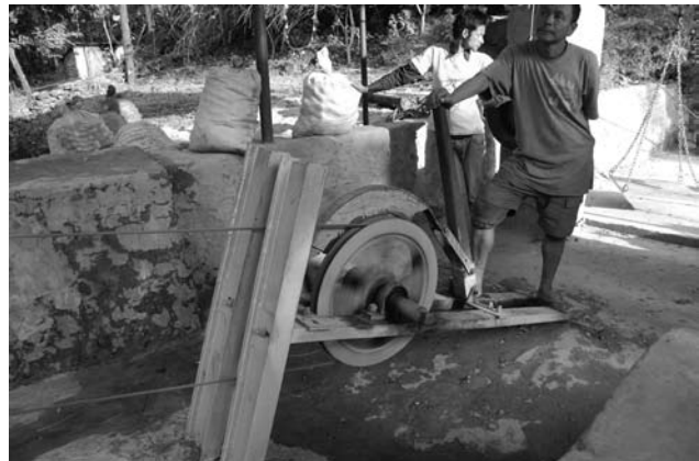
Photo 5: Ropeway operator waiting to apply brake
