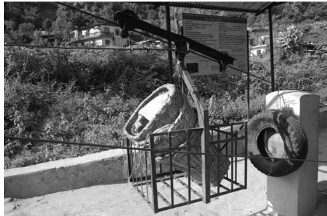
Photo 4: Example of a typical ropeway trolley
